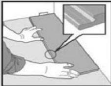
First plank, first row. Place a spacer of 15mm thickness to the left and position the plank against the wall. Later, after 3 rows, you can easily position the flooring against the front wall with distances  $\approx$  15mm.
