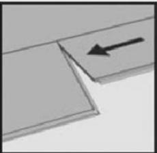
Second plank, second row place the panel at an angle into the groove of the previous row making sure that the end of the panel is tight/flush to the short end of the previous panel.
