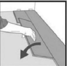
Fold the panel down in a single action movement with a slight press to the left to the short end of the previous panel. Again using the tapping block tap it against the long end into the previous row. During the fold down, make sure the panels are tight against each other.
