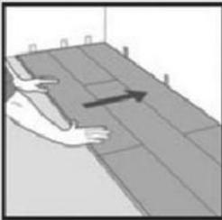
After 2-3 rows, adjust the distance to the front wall by placing spacers  $\approx 15\text{mm}$ . Once the adjustment is done against the main wall, continue to install till the last row.
