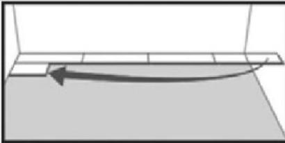
General distances between short ends. Minimum distance between short ends of planks in parallel rows shall not be less than 500mm. This is for stability of the floor.
