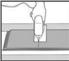
Cut with a jig saw - hardwood turned down to eliminate/reduce damage to the face of the panel. Or if cutting using a hand saw, cut it with the hardwood visible face up. Then install it as previous plank.
