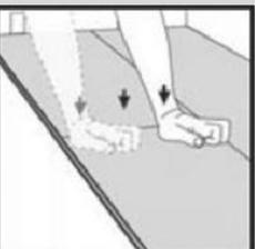
As it flattens itself to the floor, press or gently tap the top of the short end of the installed panel until it clicks. Finish installing this plank by tapping it with a tapping block on the long side to ensure secure installation.
