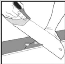
Installation at radiators. Drill the holes 20mm larger than the diameter of the pipes. Cut out the panel (with the thinnest blade possible) as per diagram. Install the plank as per normal. Glue the cut out piece back again.
