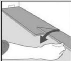
Fold the panel down in a single action movement. During the fold down, make sure the panels are tight against each other. Afterwards press down or slightly tap down at the short end just installed till it clicks. No major force is required.
